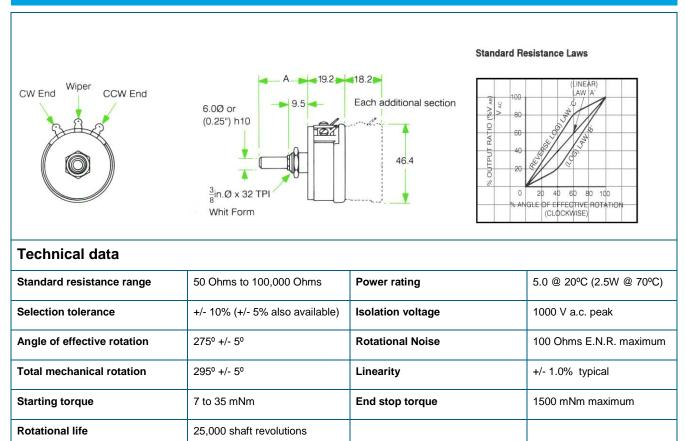
High quality, general purpose wirewound panel control of robust and reliable construction. Phenolic body moulding; nickel silver contact; nickel plated brass spindle and bush; electro-tin plated brass termination tags.
