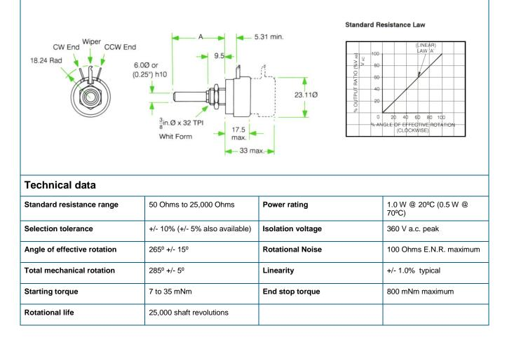
General purpose sealed wirewound panel control of robust and reliable construction. Phenolic body moulding; beryllium copper contact; nickel plated brass spindle and bush; silver plated brass tags.
