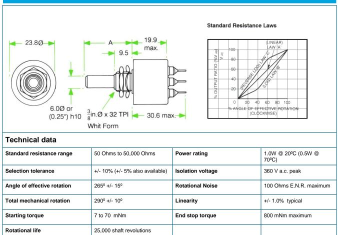
High quality container sealed, wirewound panel control of robust and reliable construction, with spindle and panel seals. Aluminium case and bushing; Anodized aluminium alloy spindle and fixing nut; nickel plated brass lid; silver plated brass tags insulated from lid by ceramic standoffs.
