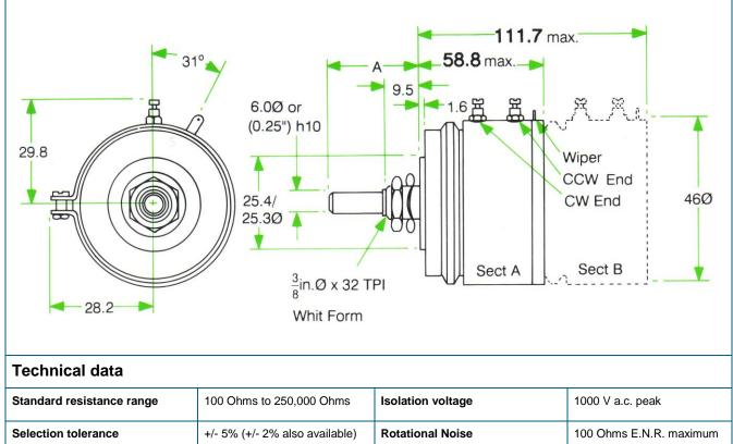
Standard resistance range100 Ohms to 250,000 OhmsIsolation voltage1000 V a.c. peakSelection tolerance+/- 5% (+/- 2% also available)Rotational Noise100 Ohms E.N.R. maximumAngle of effective rotation3600° + / - 2°Linearity (Independent)+/- 0.5%Power rating4W @ 20°C (2.0W @ 70°C)Starting torque18mNm maximumEnd stop torque800 mNmRotational life10,000 shaft revolutions
